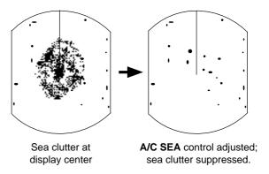
Figure 2-2 How to adjust the A/C SEA control
